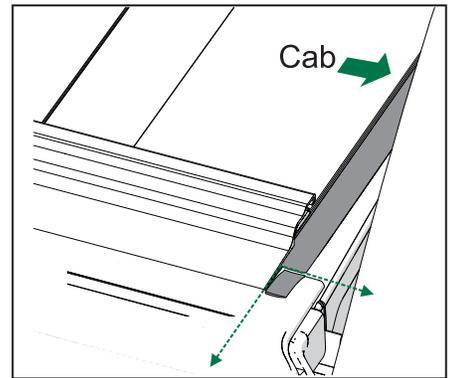
**13 Position the rails:** Move the cover back toward the tailgate and use the shipping bracket as a spacer to position both rails to be 1/8" from the tailgate.
