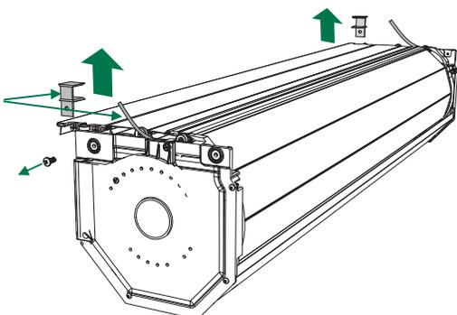
**8 Install the rails to the canister:**
