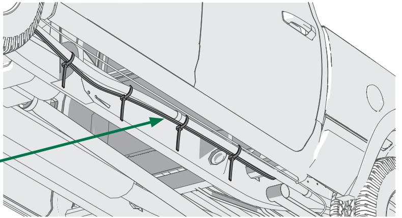
**2** Route the wire harness (D) to the driver side of the truck if it is not already. **Note: Using wire ties (E), secure the wiring harness (D) so it does not come into contact with moving parts or exhaust pipes.**
