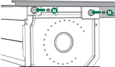
Tighten the canister mounting screws to: 32 in-lbs.
